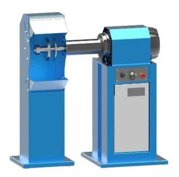
The Aceti Art 172 & Art 173 Single ended polishing lathes are extremely robust machines with twin speed motors and DC injection breaking. They have a parallel shafts as standard. An optional inverter is available for these machines that will allow the units to run between 150 & 3000 rpm. Lockable stop to prevent unauthorised use. Full guard with extraction port and eye shield included.
