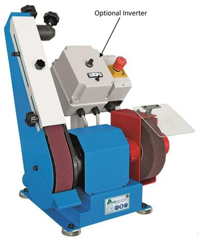
The Aceti Art 82 is a small bench mounted abrasive belt linisher and polisher. The belt arm can be orientated for the optimal working position and is fully guarded. The polisher is ideal for SCM wheels and flap wheels. The polishing head uses a parallel shaft with spacers for safety,
