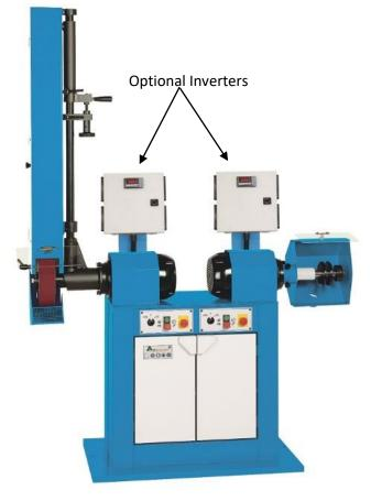
The Aceti Art 70 is an independent motor telescopic arm abrasive belt linisher and polisher. The twin motors allow for independent use of each side of the machine allowing for 2 different operations to be carried out simultaneously with the belts and polishing heads running independently.
