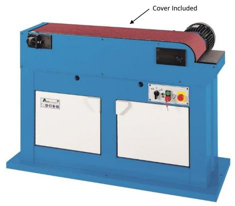
The Aceti Art 64 is a heavy duty flatbed abrasive belt linisher designed for working on large castings and fabrications. Ideal for engine blocks and housings. Perfect for giving an excellent flat surface without the expense of milling.
