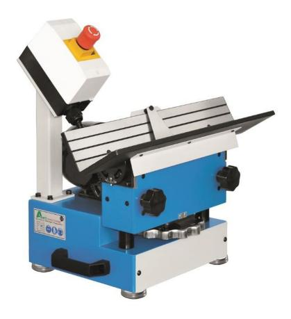
The Aceti Art 61 is a robust chamfering machine. The machine uses 10 TCT cutters to chamfer flat and box section from 15 to 45 degree angles and from 0 to 6mm chamfers.
