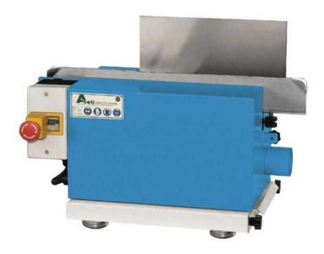
The Aceti ART 53 is an abrasive belt bench mounted deburring machine for deburring both sides of a sheet simultaneously. It has a maximum capacity of 0-2 mm flat sheet.
