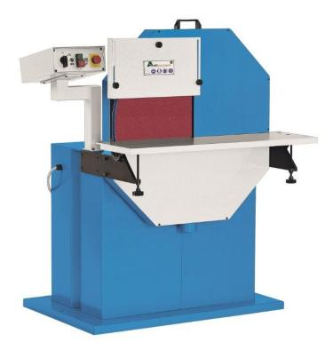
The Aceti Art 52 abrasive disc grinder is a heavy duty machine designed for the rigors of a production environment.
