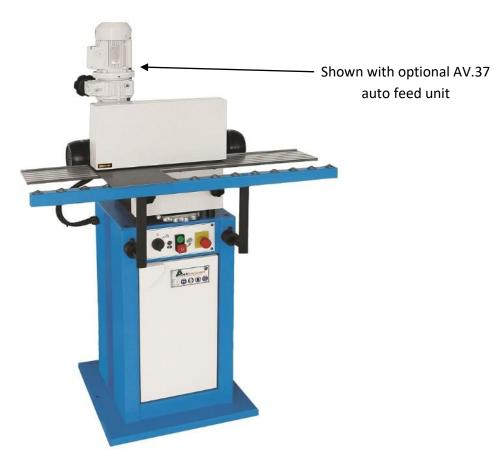
The Aceti Art 37 is an ideal machine for deburring sheet up to 4mm thickness. With the option of the AV.37 auto feed unit with variable feed speeds to allow for semi auto deburring to speed up the operation. The machine comes on a cabinet stand with low voltage electrics and DC injection braking. Supplied with 60 grit flap wheels fitted.
