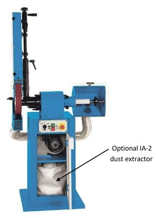
The Aceti Art 32 is a robust Telescopic abrasive belt grinder and Polisher mounted on a useful cabinet stand. The belt arm is telescopic so can accept belts from 2000 to 2500mm in length. The arms orientation can also be adjusted to suit the work required. The polishing side will accept all mops up to 250mm dia with a parallel bore of 25mm.
