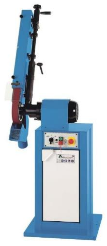
The Aceti Art 28 is a robust abrasive belt grinder mounted on a useful cabinet stand. The belt arm is telescopic so can accept belts from 2000 to 2500mm in length. The arms orientation can also be adjusted to suit the work required
