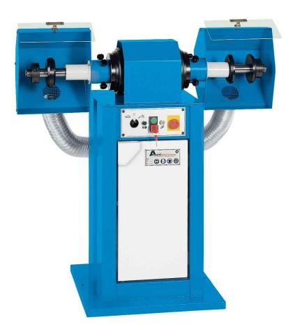
The Aceti Art 27 & Art 46 double ended polishing lathes are extremely robust machines with twin speed motors with DC injection breaking. They have a parallel shafts as standard. An optional inverter is available for these machines that will allow the units to run between 150 & 3000 rpm. Lockable stop to prevent unauthorised use. Full guard with extraction port and eye shield included.
