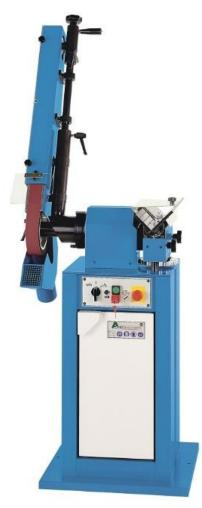
The Aceti ART 23 is a robust telescopic arm abrasive belt linisher and chamfering machine mounted on a useful cabinet stand. The head can be orientated for the optimal working position. The chamfering machine uses 10 TCT cutter to chamfer flat and box section from 15 to 45 degree angles and from 0 to 6mm chamfers.
