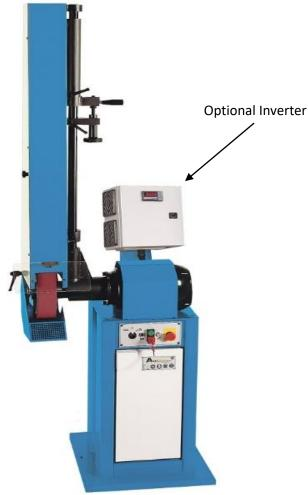
The Aceti ART 128 is a telescopic arm abrasive belt linisher. The belt arm can be orientated for the optimal working position and is fully guarded.
