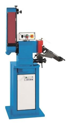
The Aceti 104 Drill sharpener and Abrasive Belt Linisher is a heavy duty machine designed for the rigors of a production environment. The unit has low voltage controls and a twin speed motor for better control Suppled with cabinet stand for handy storage
