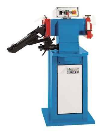
The Aceti 102 Drill sharpener and abrasive wheel grinder is a heavy duty machine designed for the rigors of a production environment. The unit has low voltage controls and a twin speed motor for better control Suppled with cabinet stand for handy storage
