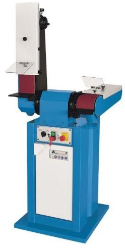
The Aceti ART 08 is a robust twin arm abrasive belt linisher designed for use on both the contact wheel and platen. Mounted on a useful cabinet stand. The arms can be orientated for the optimal working position. Low volt controls and DC injection braking are supplied as standard.
