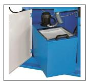
The Aceti Art 65 centreless can cope with all tube sizes from 5 to 110 mm. It has a twin speed belt motor allowing for speeds of 18 and 36 M/s. (1400 / 2800rpm). The machine comes equipped as standard with a coolant pump for wet use.
