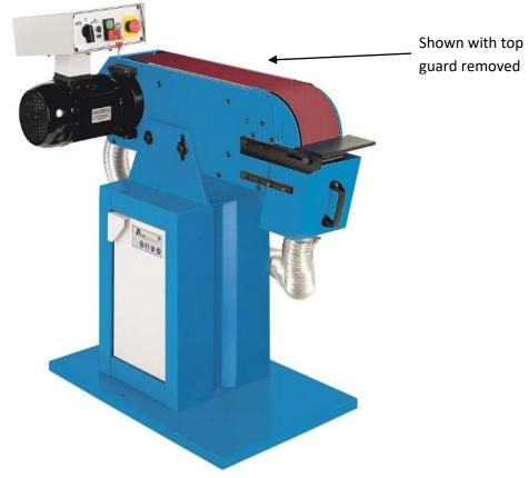
The Aceti Art 38 is a "Heavy Duty" abrasive belt grinder mounted on a useful cabinet stand. The head can be raised and lowered for the optimal working height.
