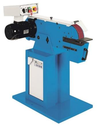
The Aceti Art 33 is a "Heavy Duty" abrasive belt grinder mounted on a useful cabinet stand. The head can be raised and lowered for the optimal working height.
